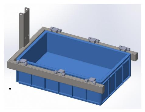
3. Locking cams rotate as tool is lowered
