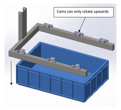
2. Locking cams contact crate, lower tool further
