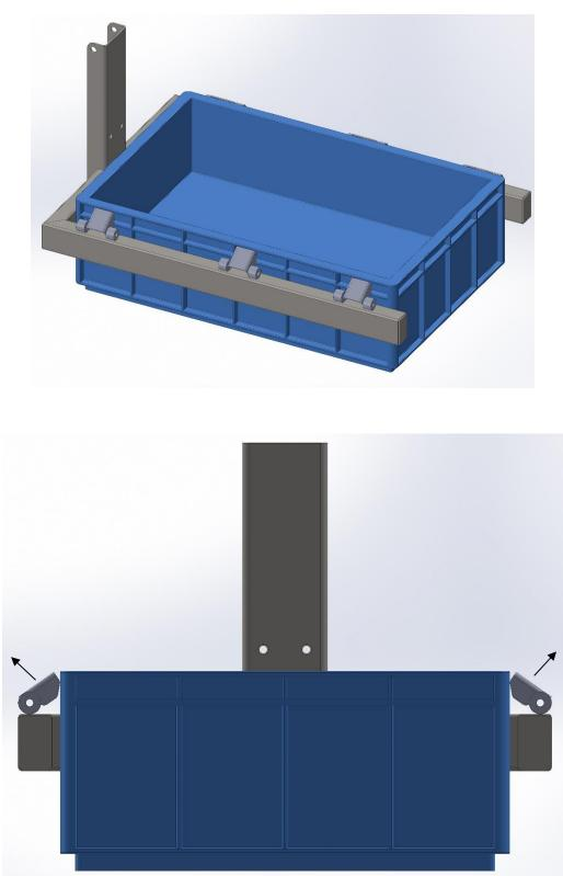
4. Cams drop into locked position, crate can now be lifted
